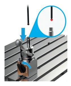
Mount the ACS-1 on the multi-tasking lathe.
