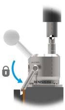
**CAUTION:** Once the plunger has been set in position using the locking lever, do not depress the plunger again until calibration has been completed and the locking lever has been released. The plunger provides 10 mm (0.39 in) of travel. Damage to the unit can occur beyond this point.
