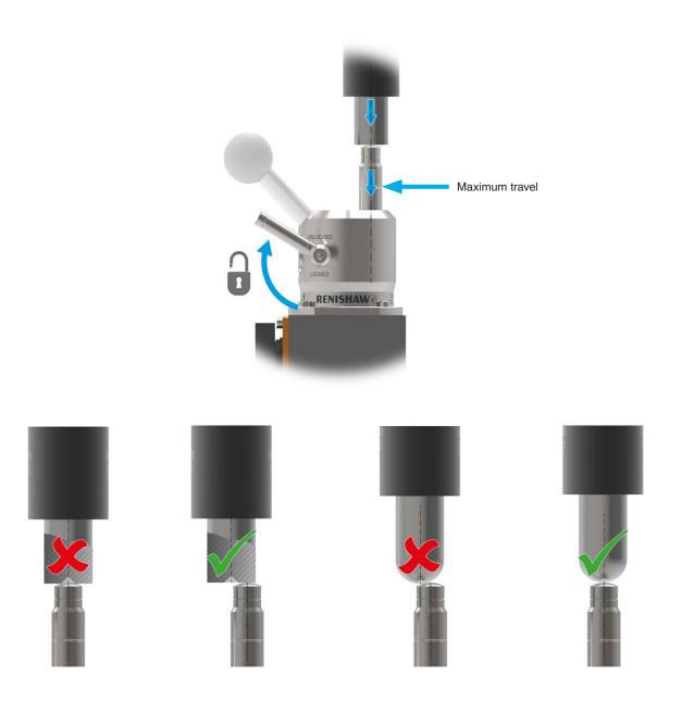
2. The lever can now be locked and a machine datum set in Z.
