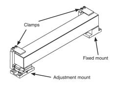
Figure 7: mirror clamped in mount
