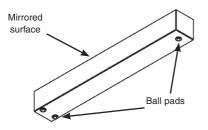
Figure 3: mirror with ball pads
