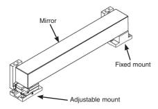
Figure 4: mirror located in mounts
