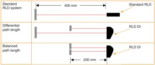
Figure 2 below shows a schematic of the various optical configurations tested.
