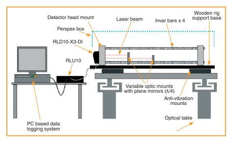
Figure 4: test rig set-up
